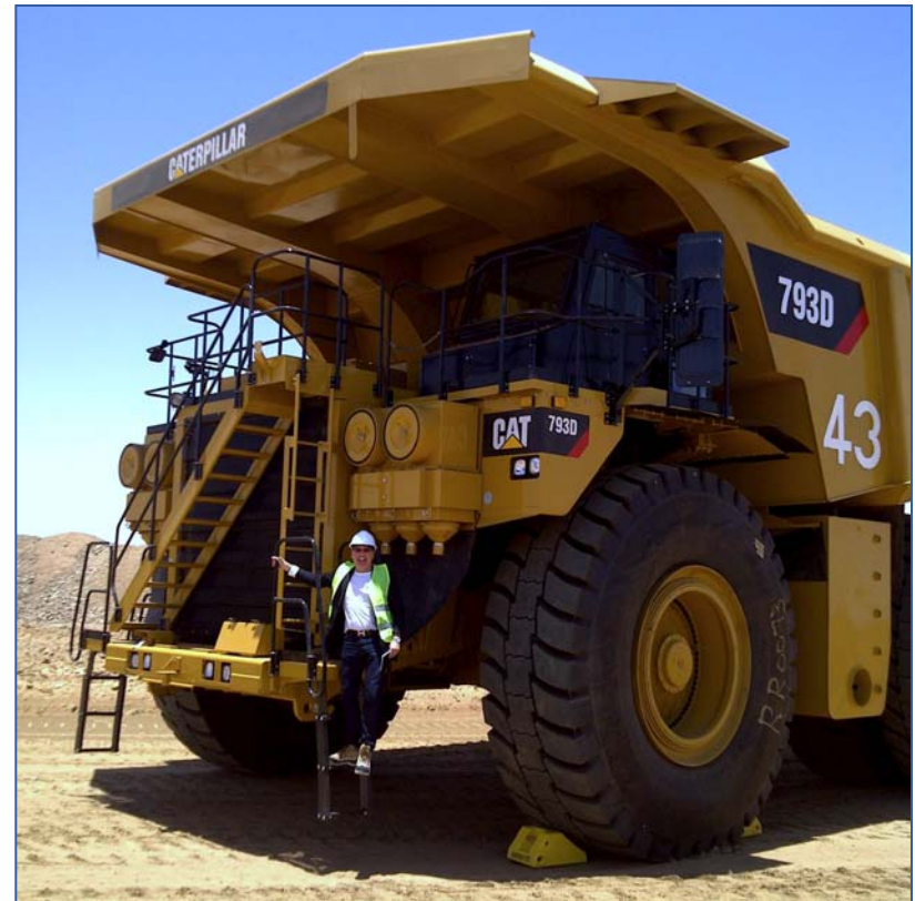
Weight of Truck: 423 tons Load Capacity: 240 tons
